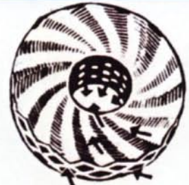
View showing level-by-level construction of Wound Cartridge
